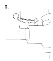
Please note: The top graphic fixing loop must be facing down and the bottom graphic loop fixing must be facing up
